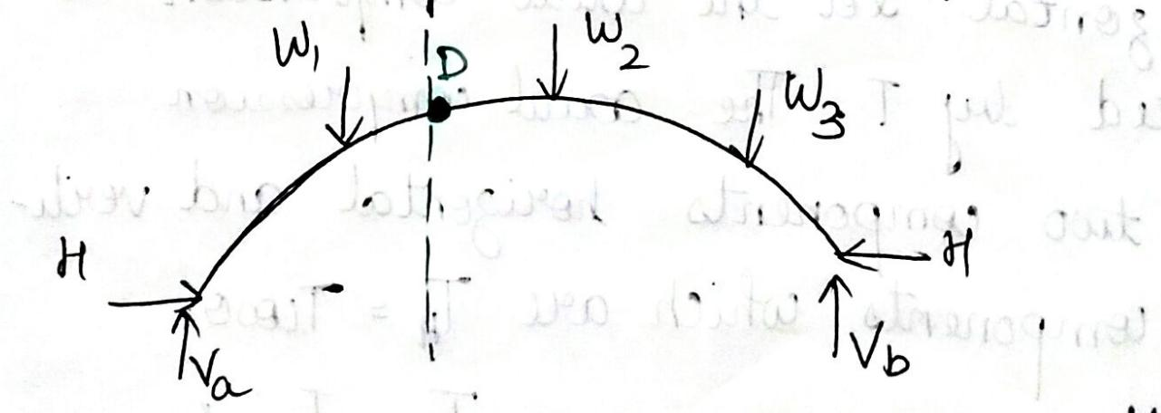
At that point horizontal thrust, and Net vertical shear,  $V$  will be acting
